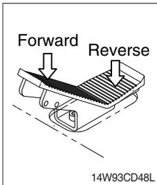
(1) This pedal is used to select traveling direction and to accelerate of the machine.
