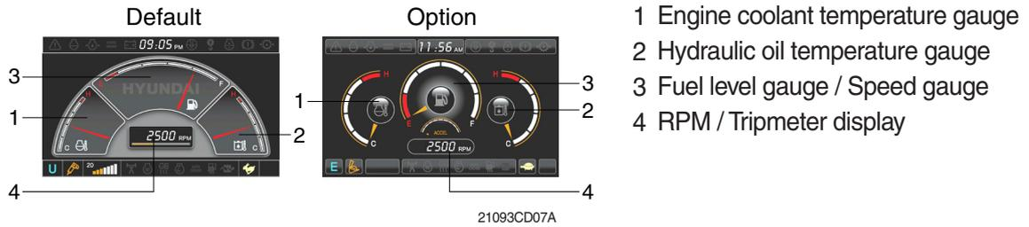
※ Operation screen type can be set by the screen type menu of the display.
