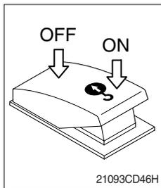
(1) When this switch turned ON, buzzer makes sound and overload warning lamp comes ON in case that the machine is overload.
