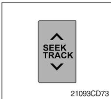
① If this button pressed, the radio automatically stops at the next frequency of broadcasting for your listening.
