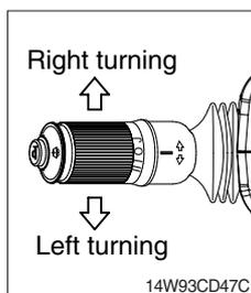
① This switch is used to warn or signal the turning direction of the machine to other machines or equipment.
