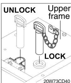
(1) This is the system to lock the swing by connecting the upper swing part and the lower frame mechanically.
