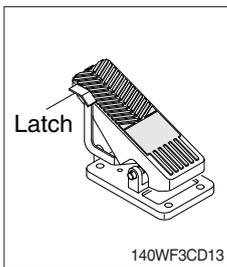
(1) Pedal and latch provide two kinds of service brake function.
