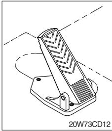
(1) When this pedal is stepped, the machine starts traveling.
