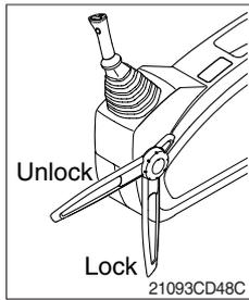
(1) All control levers and pedals are disabled from operation by locating the lever to lock position as shown.
