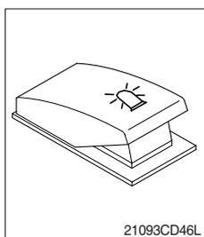
(1) This switch turns ON the rotary light on the cab.
