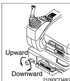
(1) This lever is used to move the LH and RH control lever to fit the contours of the operator's body.
