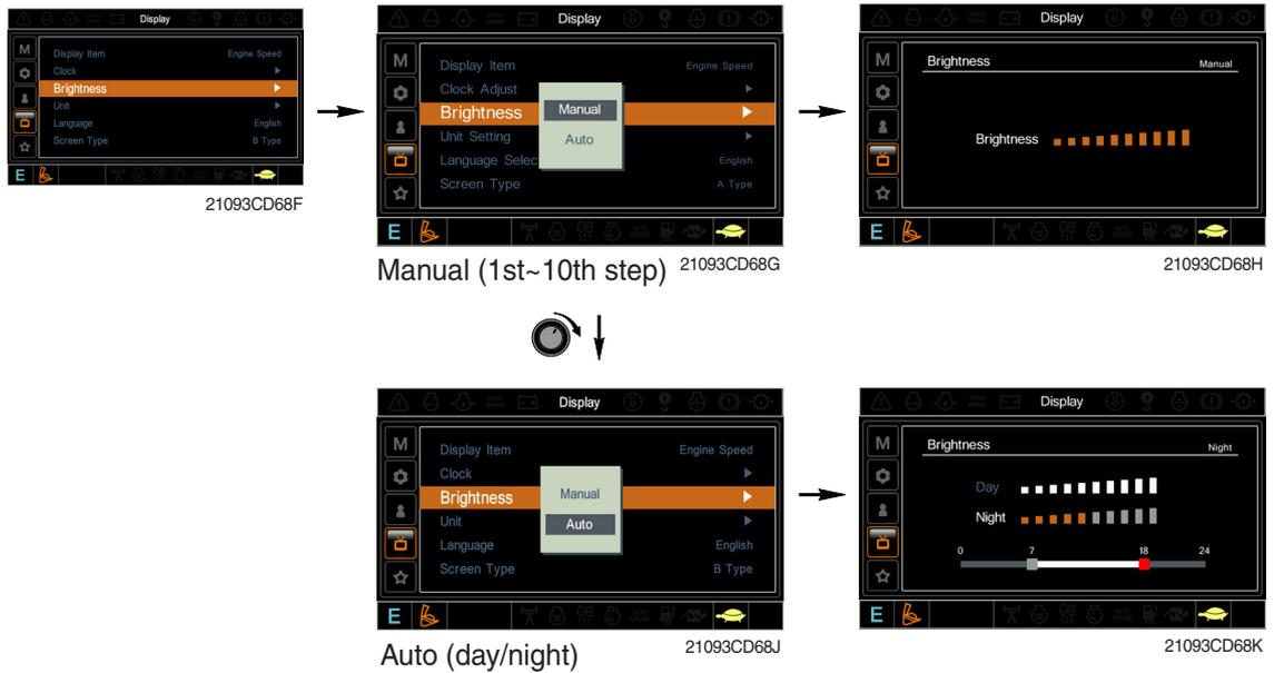
※ If "Auto" is chosen, brightness for day and night can be differently set up. Also by using the bar in lower side, users can define which time interval belongs to day and night. (in bar figure, gray area represents night time while white shows day time)
