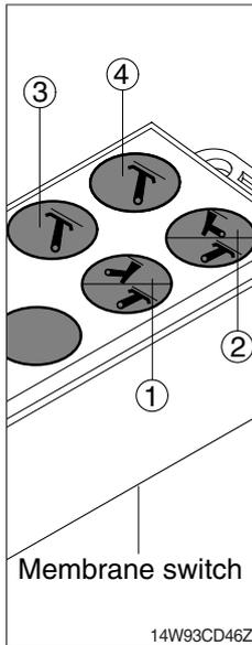
(1) This switch is used to select dozer blade or outrigger operation.
