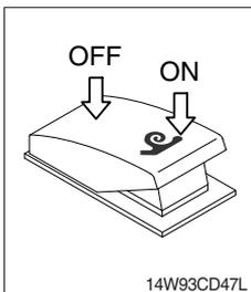
(1) This switch is used to very low speed traveling more than 1st speed.
