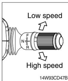
① This switch is for selecting travelling speed between high and low.
