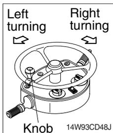
(1) If the steering wheel is turned to left, the machine will move to the left and turn it to the right, the machine will move to the right.
