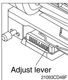
(1) This lever is used to move the seat and console box to fit the contours of the operator's body.
