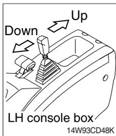
(1) This lever is used to operate dozer blade or outrigger by selecting the select switch 1 (dozer / outrigger).
