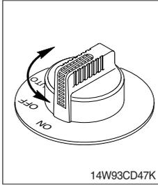
(1) This switch activate front axle oscillation cylinder to locking position for increase of stability.
