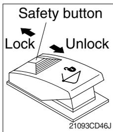
(1) This switch is used to engage or disengage the moving hook on quick clamp.
